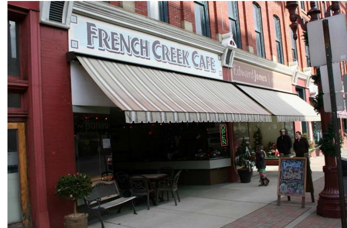
An awning can cover no more than 1/3 of the storefront and 2/3 of the sidewalk area.
